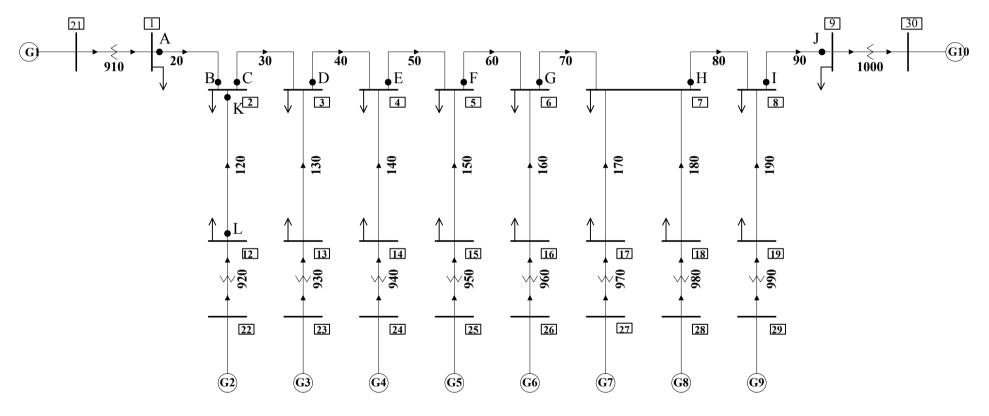
Notes: All lines in this figure represent 2 circuits of 3-phase transmission line.
