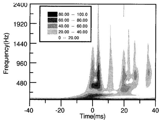
Fig. 4. The dynamic spectrum of zero-sequence current under no rain (inferior air switch).
