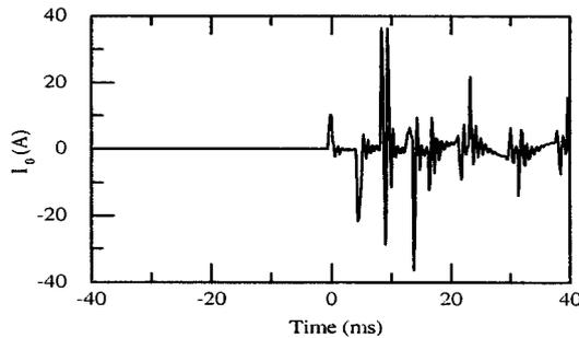
Fig. 2. An example of zero-sequence current waveform (inferior insulator and breaking of cable).
