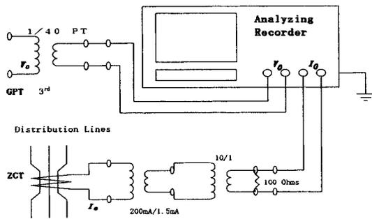
Fig. 1. A fault signal acquisition system.
