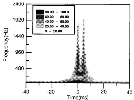
Fig. 5. The dynamic spectrum of zero-sequence current under rain (tree contacting).
