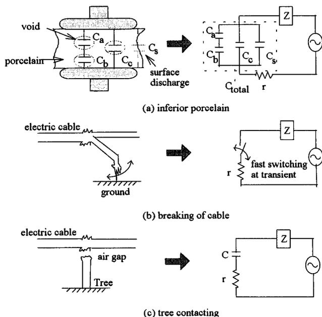
Fig. 6. The ideas and equivalent circuits at ground fault points of some cases.
