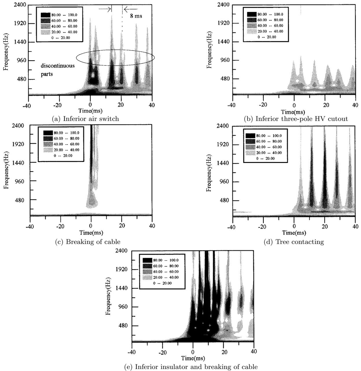
Fig. 3. Examples of dynamic spectra of zero sequence current resulting from different causes.
