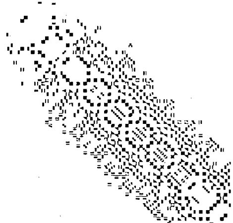
Fig. 6. The decompressed CGH using JPEG baseline decoding system (size: 257kb, 18.07 \times 18.07\text{cm}^2 , 512 \times 512\text{pixel}^2 , 8bpp/grayscale, q(N)=2 , R\% = 100\% .)
