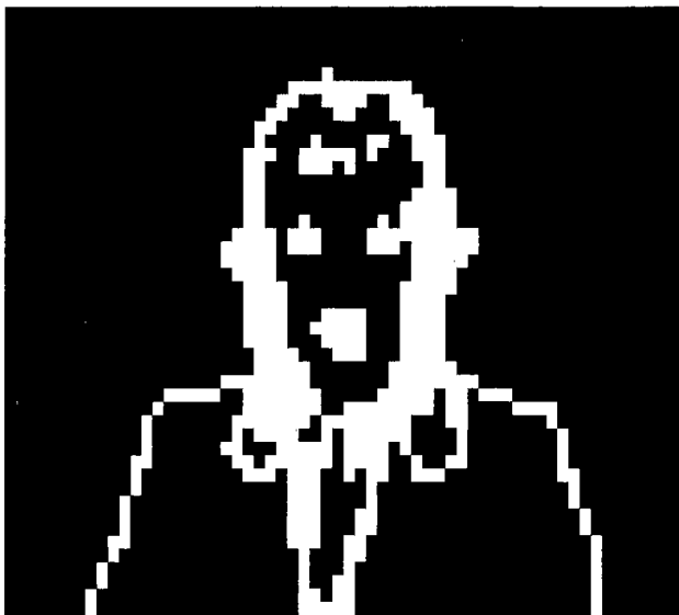
Fig. 6. The segmentation result with region growing approach based on block.
