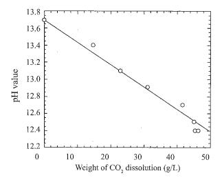
Fig. 3. pH value of TMAH solution.
