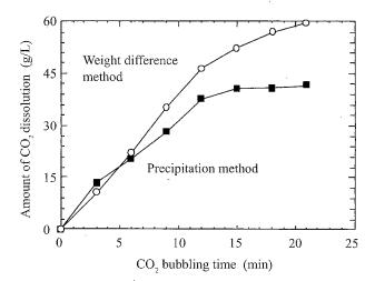
Fig. 2. Contents of CO<sub>2</sub> versus bubbling time.
