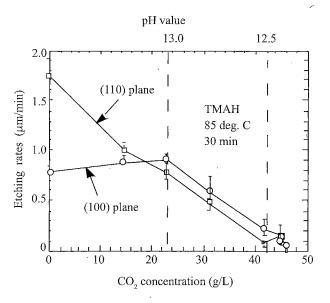
Fig. 5. The etching rates in various contents of CO<sub>2</sub> dissolution.
